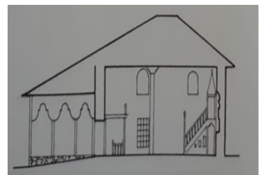
Figure 18: Mosque Section. Source: (Meksi, 2015)
